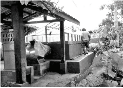
Fig. 19. An AWSD attached to a biomass furnace (1) a full-view of the facility and (2) a closer view of the furnace using available biomass materials in the area, Aurora, 2012
