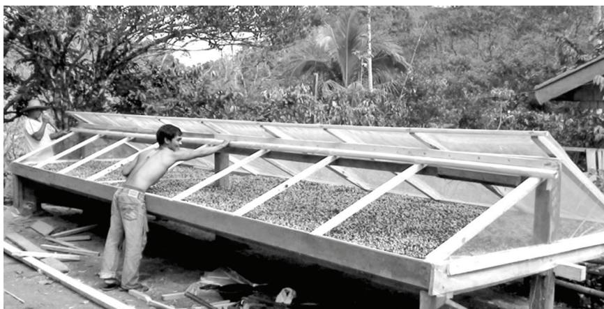
Figure 18. A farmer in Kalinga using an “AWSD” for drying depulped coffee berries, 2012
