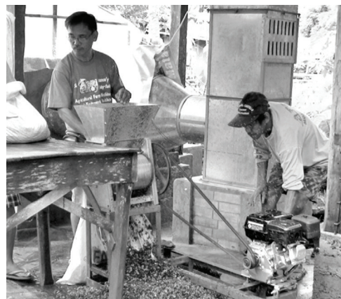
Fig. 21. A farmer in Aurora operating a coffee pulper attached to a small gasoline engine, 2012
