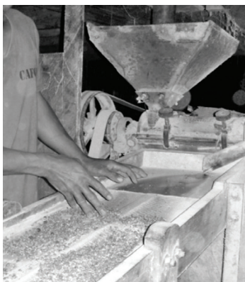
Fig. 15. Mechanical huller used for dehulling coffee, Kalinga, 2012
