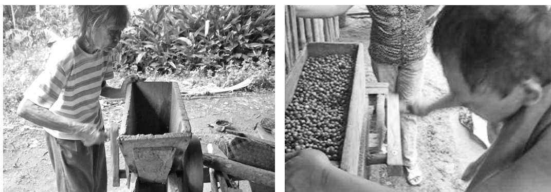
Fig. 14. Locally fabricated wooden pulper used for splitting /cracking newly-harvested coffee berries prior to sun drying, Surigao del Sur, 2012
