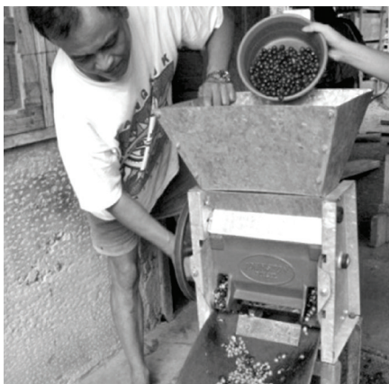
Fig. 20 . A coffee farmer in Kalinga manually operating a coffee pulper before drying his coffee in the AWSD, 2012
